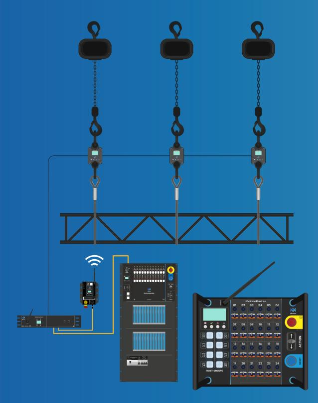
Our range of load cell monitoring system shares the same philosophy as our product portfolio of digital controllers, being able to work on choice with wired connections only, fully wireless, or a mix of both.
