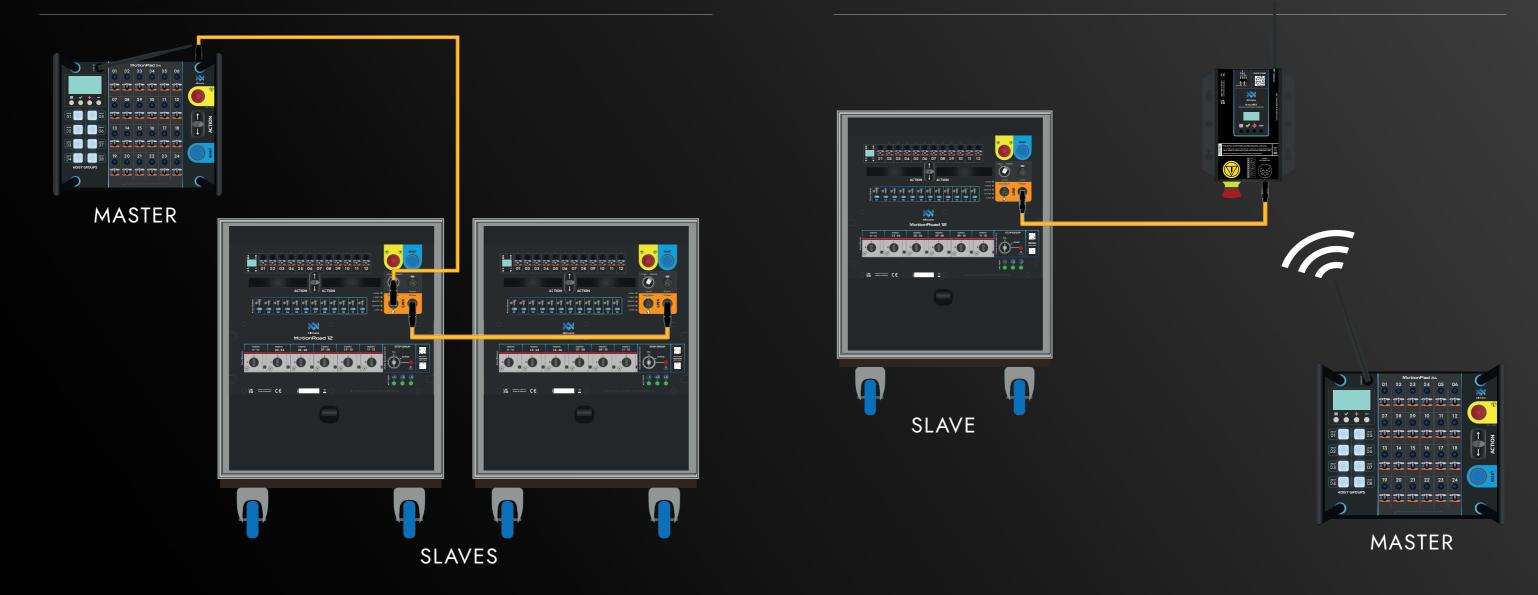
• Simply plug the cable from on controller to another. The first controller becomes a master and your system operates as one.
